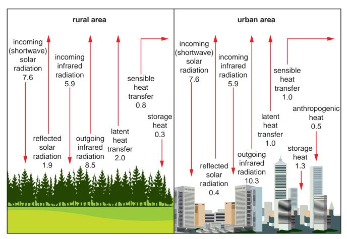
All units are in kWh/m²/day Storage heat = energy absorbed into the surface
